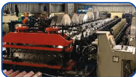
Deck Sheeting Machine
