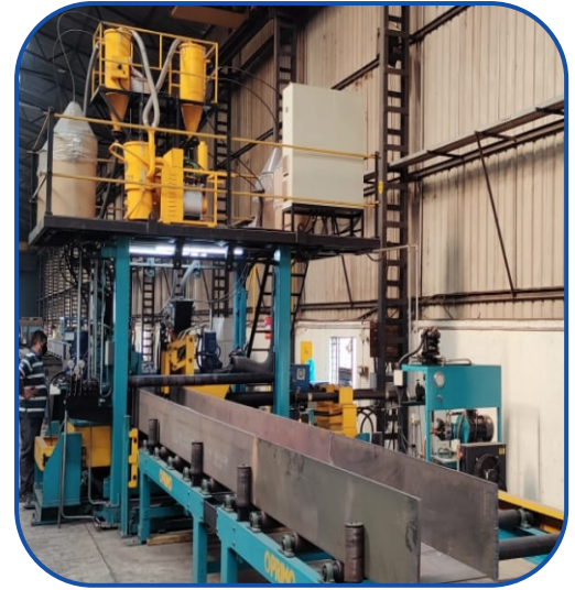
Automatic Gantry Submerged Arch Welding
